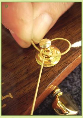
This is a half-wind to enable subsequent windings, using the tuner button, to feed onto the post BELOW the string. Cut excess string length using small end nippers or pliers. Tune string to pitch.
